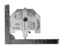
Place the gauge against the toe of the fillet weld and slide pointer out until it touches structure as shown. Read "Size of the Fillet Weld" on the face of gauge as indicated by arrow.
